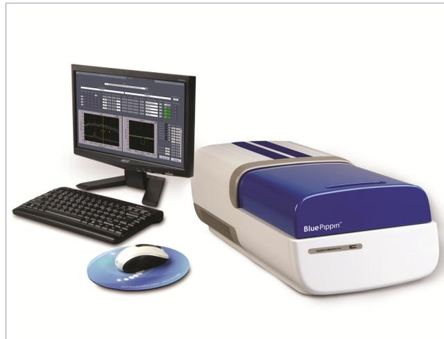
The alternating field mode allows rapid separation of high molecular weight DNA in 0.75% agarose cassettes: linear phage lambda DNA (48,500 bp) can be collected in as little as 6 hours. These features make the BluePippin useful for the size fractionation steps of mate-pair (jumping) library construction.
